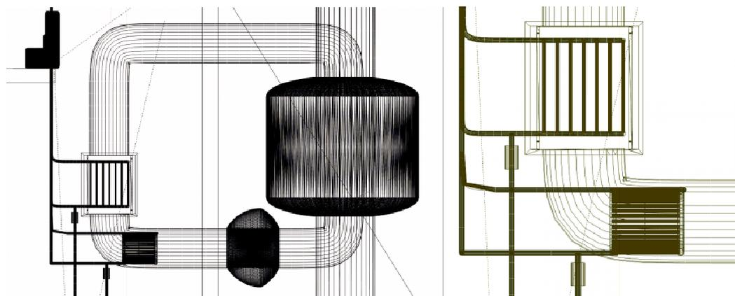
FIG. 1. DFR front view (left) and close-up of the DFR core region (right) with part of the coolant cycle and the short lived fission products storage inside the coolant conduit ahead of the core.
