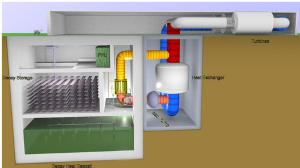
FIG. 3. Possible power plant based on the DFR. The compactness allows for a subterranean installation.
